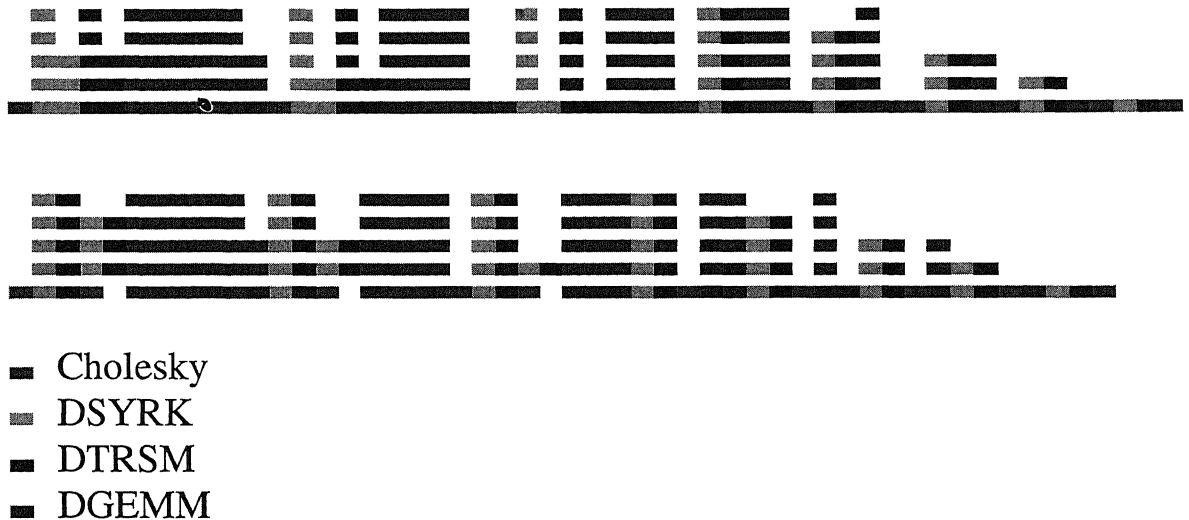
Fig. 15. Right-looking block Cholesky factorizations on five processors. The upper pattern illustrates the parallel execution of Fig. 14's implementation. A combination of DSYRK and DTRSM and the Cholesky operations can reduce idle time as is illustrated by the lower pattern.
